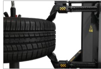
Double roller bead breakers.
