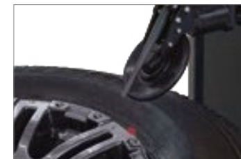
Laser pointer that indicates proper head positioning.
