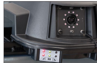
LED repeater for guided measurements without monitor.
