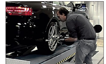
3 point + quick locking system for quick setup.
